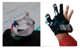
Figure 3. Left Fingers Ring version, Right Fingers 4 LEDs version
